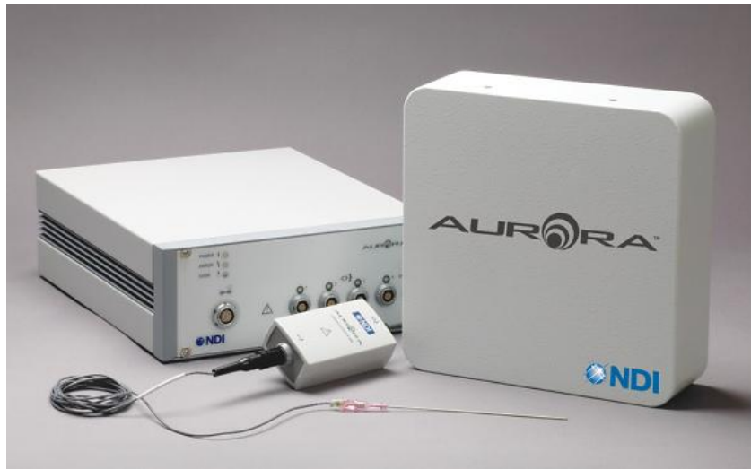
Figure 3: The Aurora magnetic tracker system from NDI[ http://www.ndigital.com/ ]
