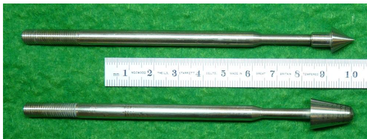
Figure 15. Test articles for experiment. Cone model (top) and blunt nose model (bottom). Each test article is attached to a 110 mm sting.
