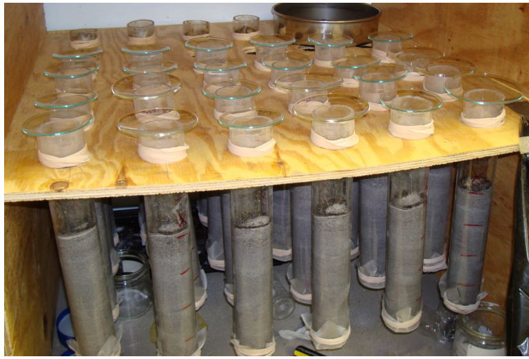
Figure 3. Experimental setup for mesocosm studies. To simulate burial, columns were hung level to soil surface and the lower portion of the wood box was covered in dark plastic to shield from light. Light was controlled in 12-hr light/dark cycles with a full spectrum light attached to the top of the box.
