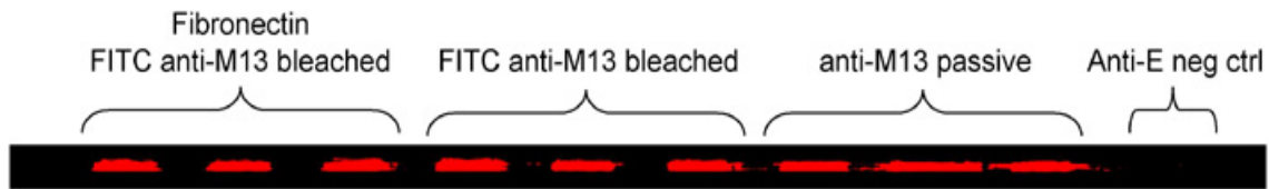
Figure 23: Virus Detection results using bleached filament. Passively adsorbed anti-M13 regions appeared less defined than bleached regions. The presence of fibronectin in bleached regions did not appear to have an effect. Average fluorescence intensity from the three different treatments was similar.
