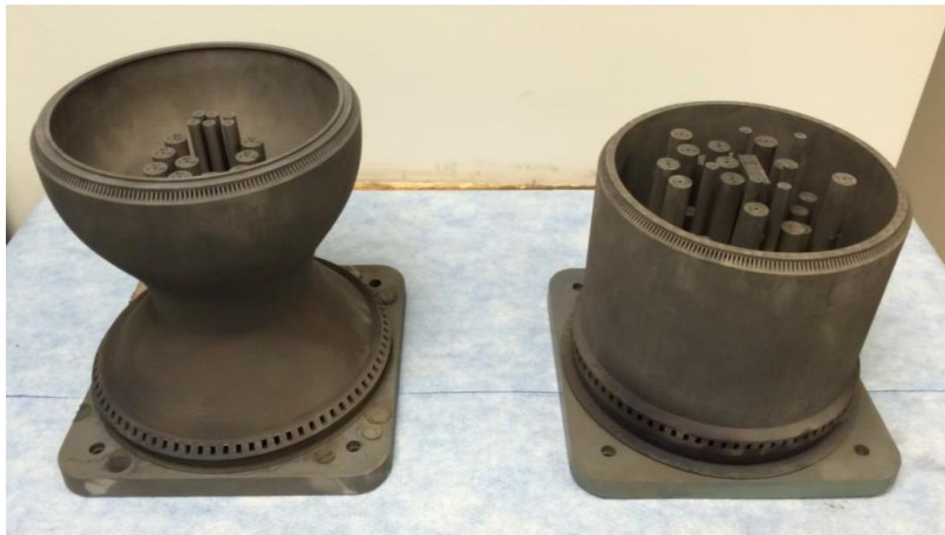
Figure 3: Bipropellant combustion chamber printed using SLM [2]
