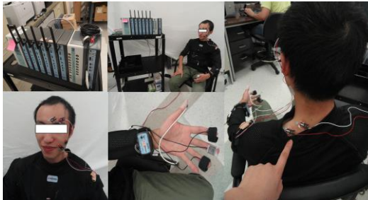
Fig. 34. Peripheral physiological electrodes placement.
