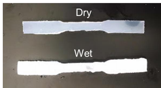
Figure 9.A7 A series of photographs showing the dissolution of a polyethylene oxide (PEO) / 1-ethyl 3-methyl imidazolium tetra fluoroborate (EMIBF 4 ) polymer electrolyte in water.
