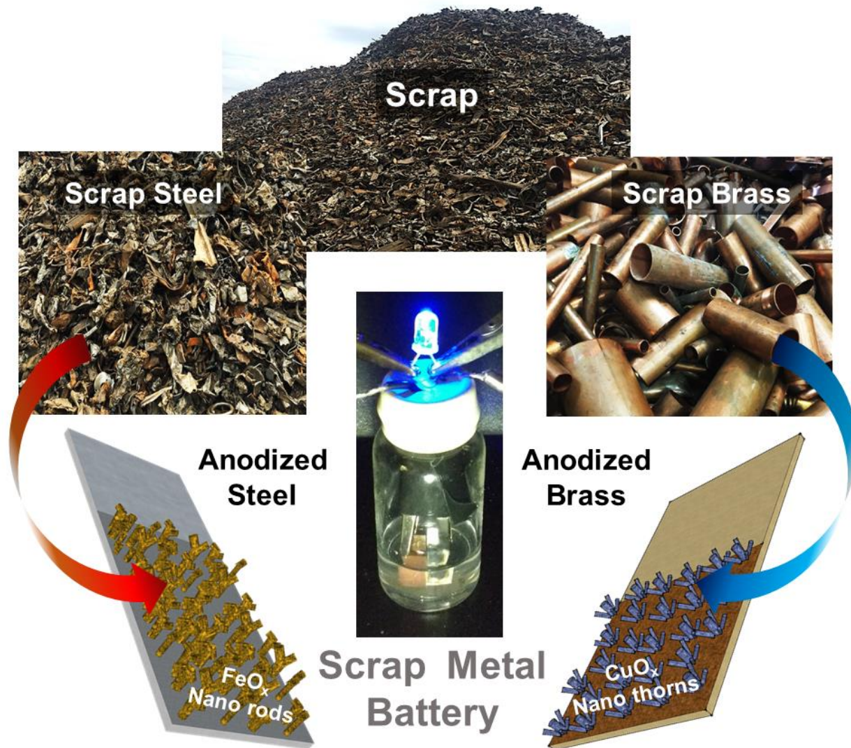
Figure 6.1 Schematic representation of the process of developing the scrap metal battery with a photograph of one of two scrap metal jar batteries powering a blue LED.
