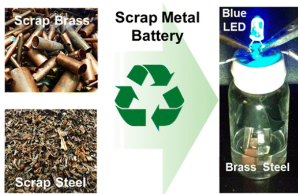
Figure 1.2 Concept of using scrap metals for batteries is depicted with pictures of scrap brass and scrap steel on the left and the picture of a full cell scrap metal battery charging an LED on the right.
