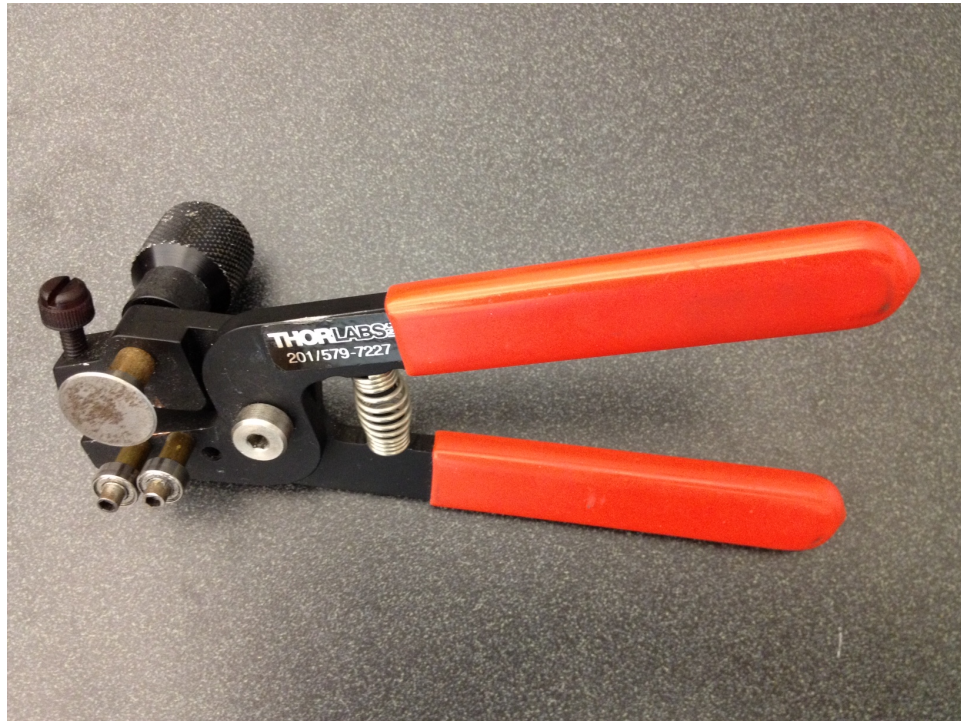
Figure V.3: A specialized tool known as a can opener used to mechanically decapsulate TO packaged devices.
