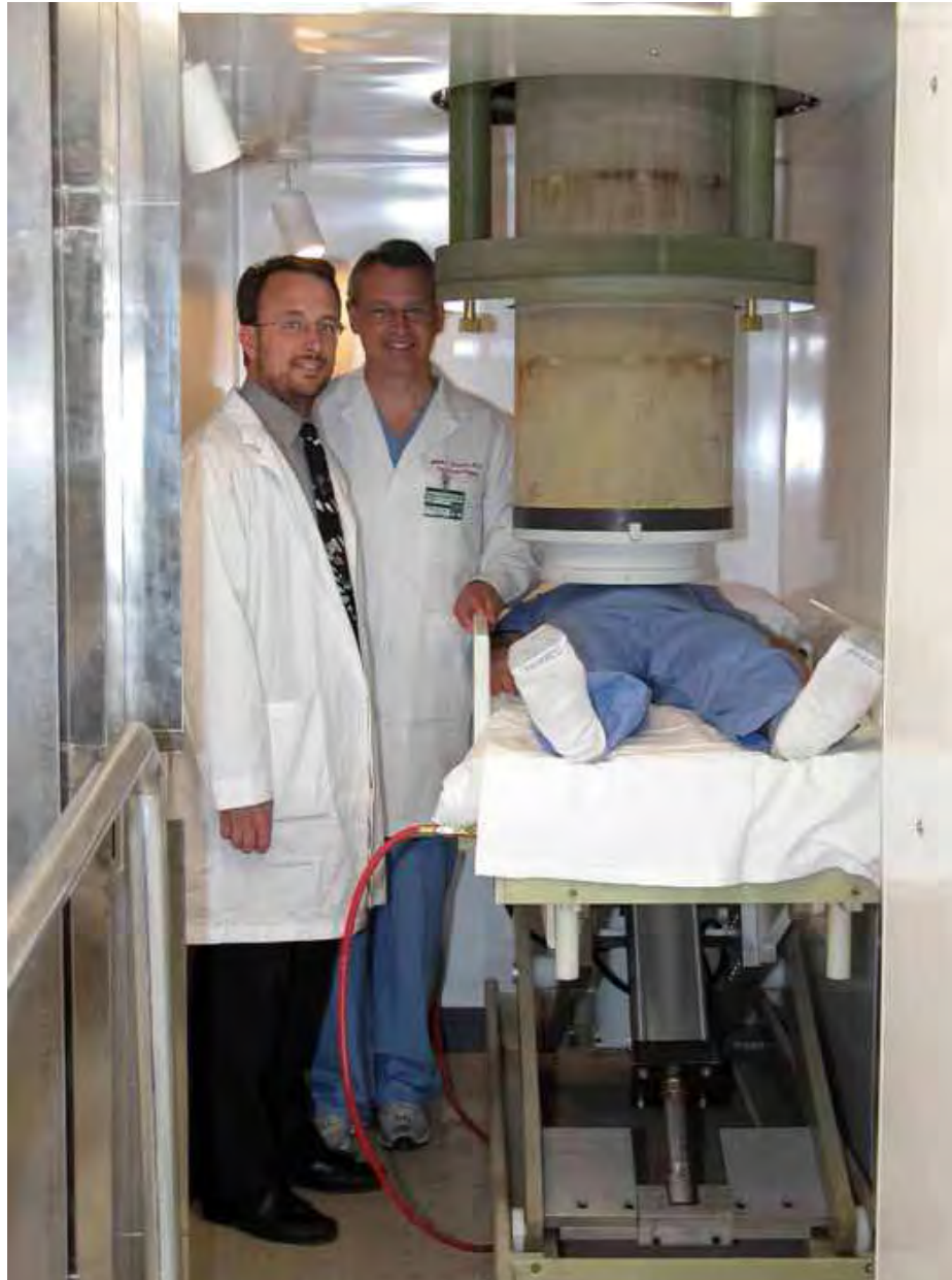
Figure I.2: The Tristan 637i SQUID magnetometer in the Biomagnetism Laboratory at Vanderbilt University. The magnetometer is located in a magnetically shielded room where measurements are taken noninvasively.
