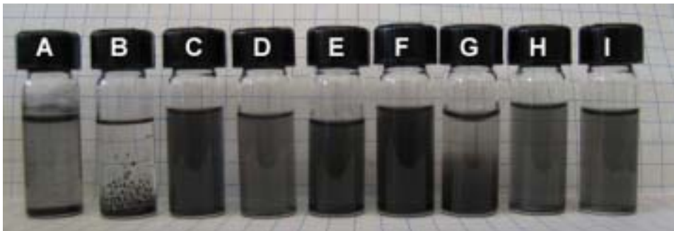
Figure 81. Dispersibility test of GCNF-CO 2 H in A) Toluene, B) Chloroform, C) Isopropyl alcohol, D) Methanol, E) THF, F) Ethyl acetate, G) Water, H) Acetone, I) DMF at the concentration of about 0.1 mg/mL
