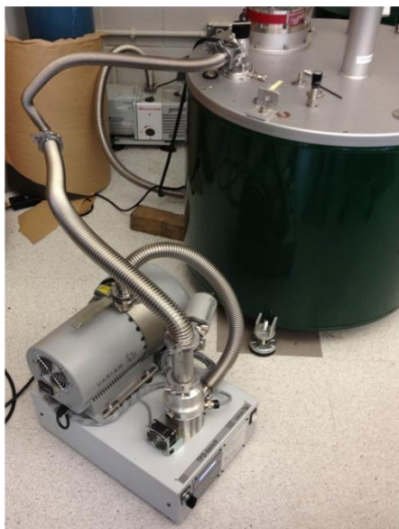
(a) Pumping outer jacket
