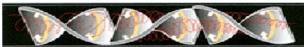
Figure 8-1. Schematic of Kenics mixer geometry.
