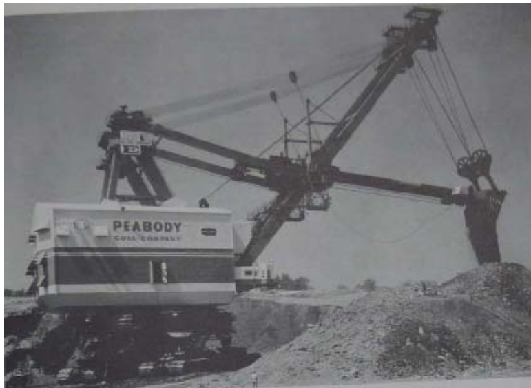
Figure 6.6: Peabody's Big Hog – A picture of Big Hog, the massive dragline that Bucyrus-Eerie built for Peabody's Sinclair Mine (for a sense of scale, see man in foreground, center). Source: TVA, The Paradise Steam Plant: A Report on the Planning, Design, Construction, Costs, and First Power Operations of the Initial Two-Unit Plant, Technical Report No. 37 (Knoxville, TN: TVA, 1964), 19, copy in NARA-SE, RG 142, OEDC, Box 636.
