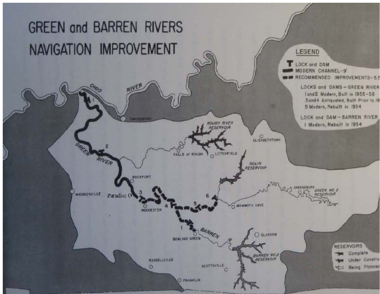
Figure 6.3: The Green River Watershed – A map of the Green River and its tributaries, including dams and locks, completed and planned, circa 1960. Source: Barren River Development League, “Report Urging Reconstruction of Locks and Dams Nos. 3 and 4, Green River, and Extension of 9-Foot Navigation Channel to Bowling Green, Kentucky,” in “Green and Barren Rivers Navigation Improvements,” March 15, 1960, 14, UKSCL, JSC, Box 40, Folder Army Corps of Engineers, Barren River Reservoir, 1956-1964.
