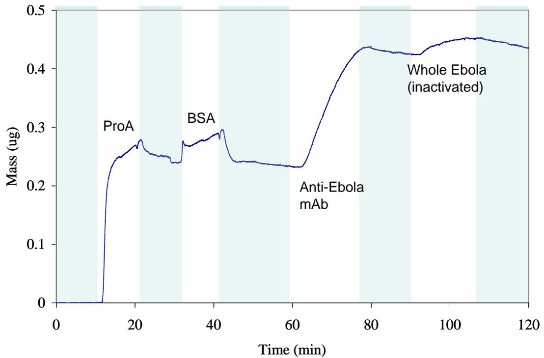
Figure 29. The QCM gravimetry shows the binding of whole ebolavirus to the EB-MAB1 antibody immunosensor. The blue regions are buffer flow only. The Ebolavirus sample was  $8.5 \times 10^4$  PFU.
