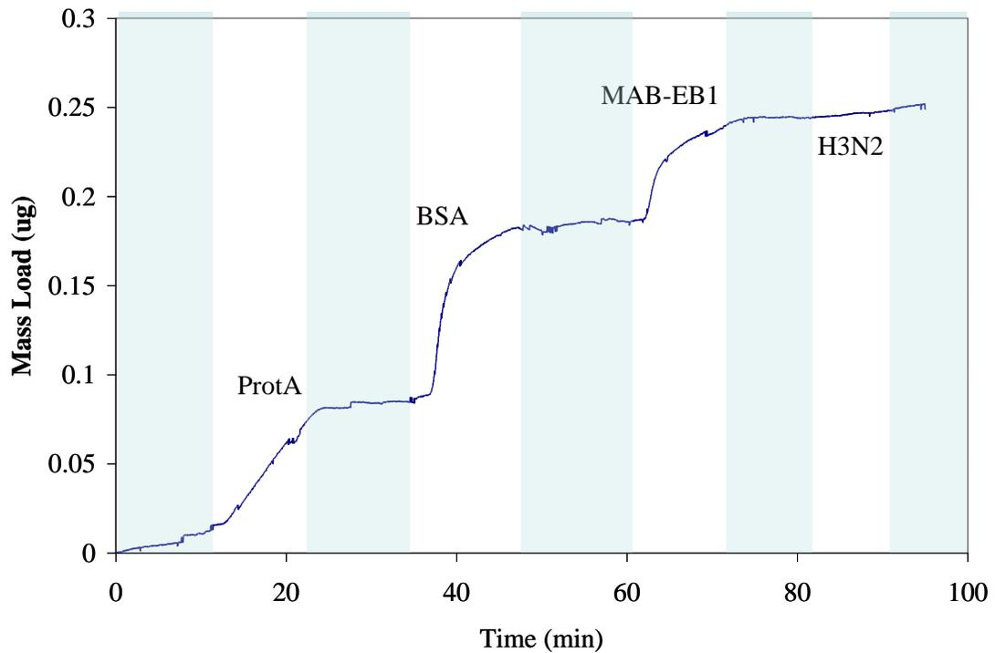
Figure 31. A second control experiment showing that the sensor does not bind another selected antigen, H3N2 flu. The EB-MAB1 shows that it has no specificity toward this antigen by the lack of H3N2 binding to the surface.
