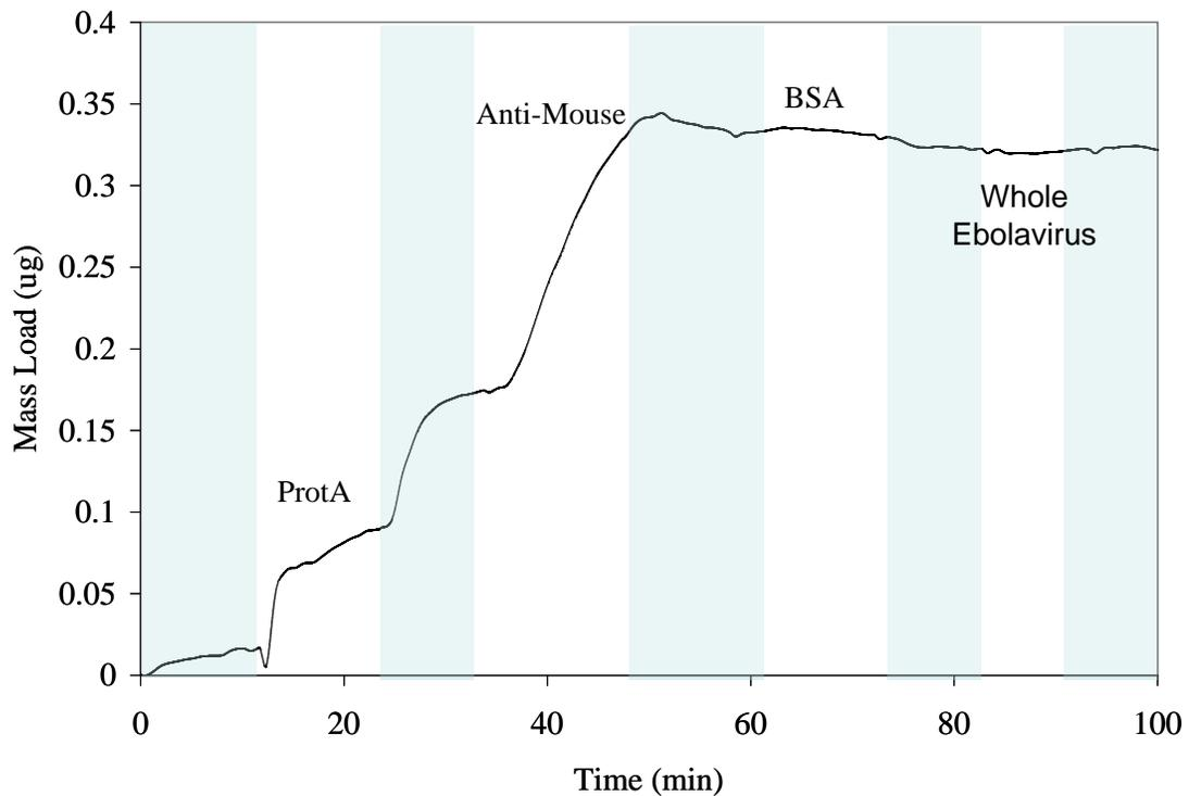
Figure 30. A control experiment showing an anti-mouse IgG based biosensor to prove ebolavirus specificity. The whole virus does not bind the sensor without the EB-MAB1 antibody.
