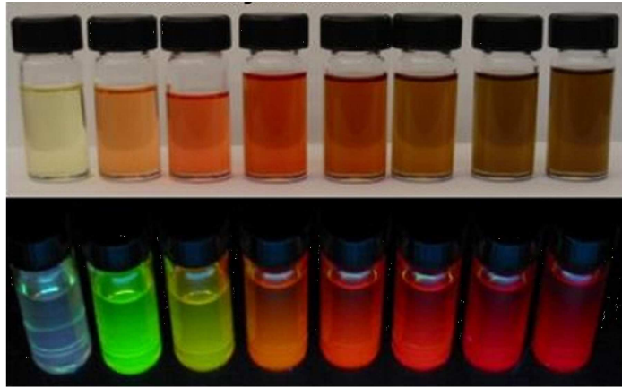
Figure 1.1: Size-dependence of the optical properties of CdSe nanocrystals. (Top) light absorption by nanocrystals ranging from small (left) to large (right). (Bottom) the same nanocrystals, illuminated by ultraviolet light, displaying size-dependent light emission. Courtesy of Michael Bowers of the Rosenthal group.
