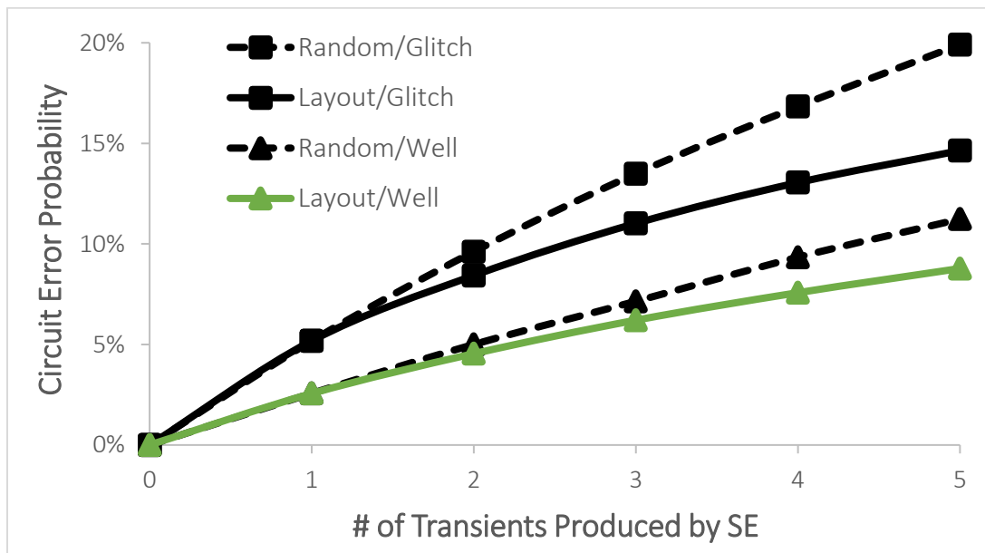
Figure IV-3. Comparison of SEMT simulation methods on the ISCAS85 circuit c3540. An average error rate for the circuit is shown using each method of glitch injection or high/low injection, using layout information for adjacency selection or random selection.
