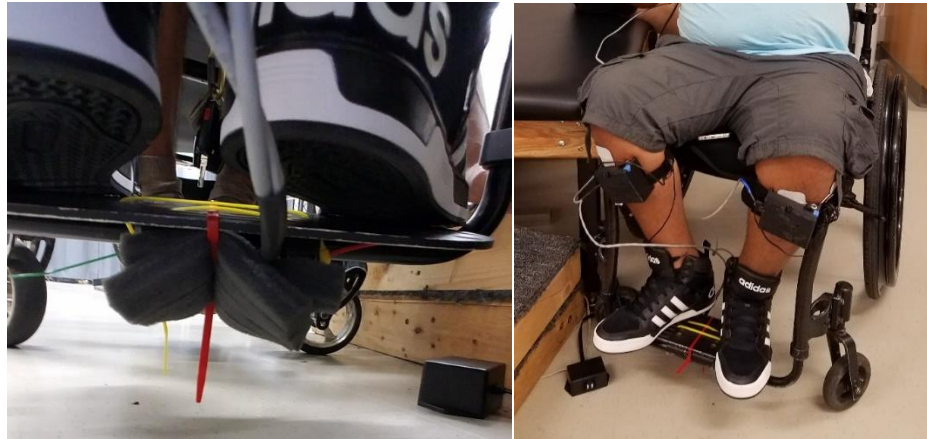
Figure 5-5: Three Chimera devices mounted on the wheelchair frame for the footrest inertia and on the lower legs for the over-ground clonus study
