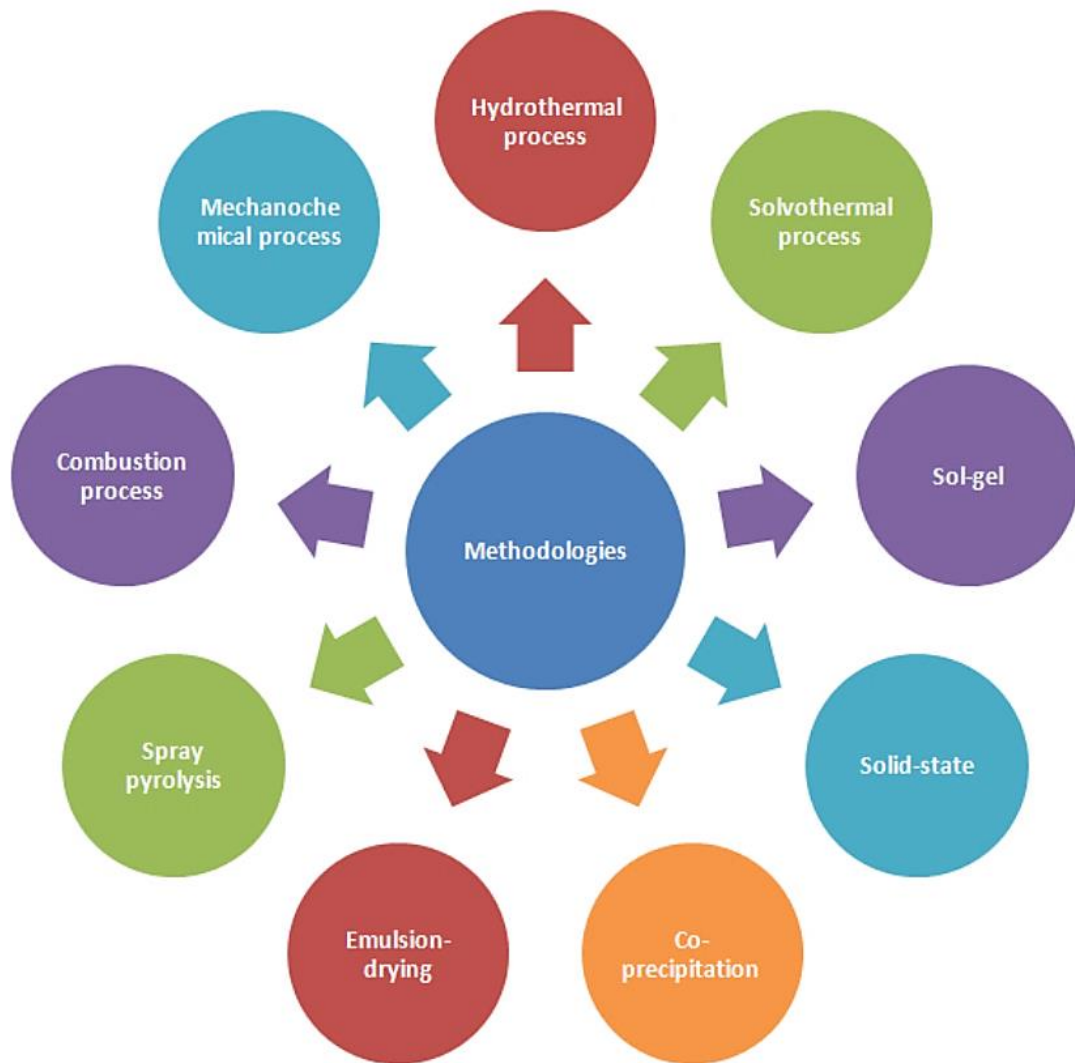
Figure 2.11 Common synthesis methods for the fabrication of cathode materials 95 .
