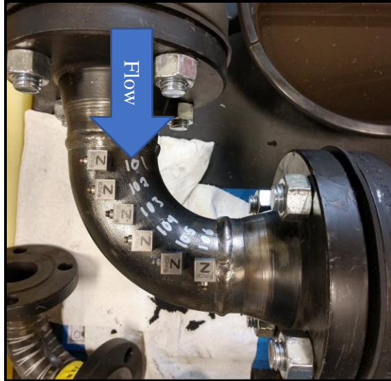
Figure 3-30: Configuration of second elbow used in mass removal experiment
