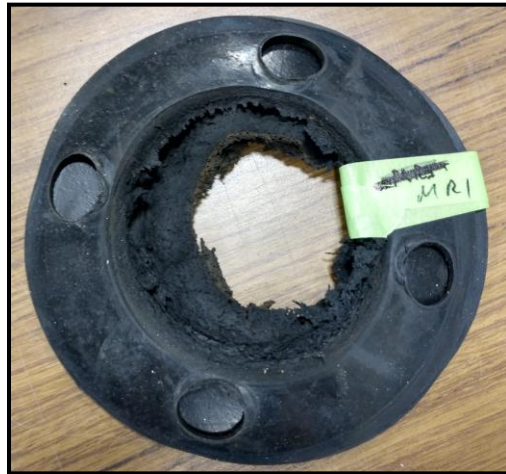
Figure 3-29: Degraded gasket after use in first mass removal experiments
