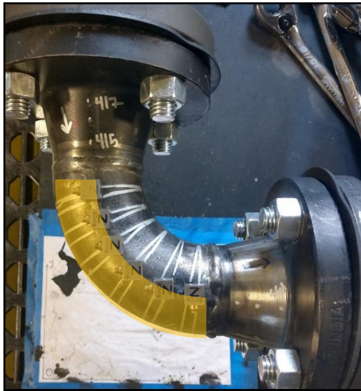
Figure 3-12: Top view of elbow with area of mass removal shown in yellow
