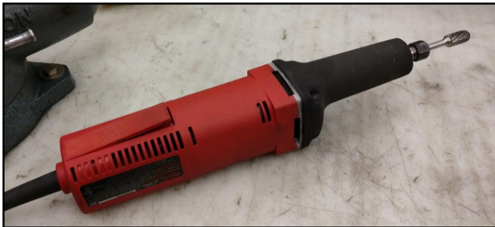
Figure 3-15: Milwaukee 2" die grinder and carbide bit used to remove material
