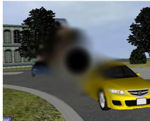
Figure V.3: Macular Degeneration simulation (a black area, 10^\circ of visual angle, surround by a blurred area, 20^\circ of visual angle).
