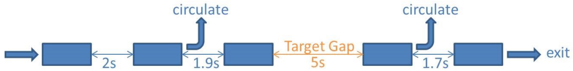
Figure IV.5: An example of an updated traffic scenario. Blue rectangles represent vehicles moving from left to right. Vehicles 1, 3, 5 will exit and vehicles 2, 4 will circulate. A target gap is randomly set between the 2nd and the 3rd car for 5 seconds.
