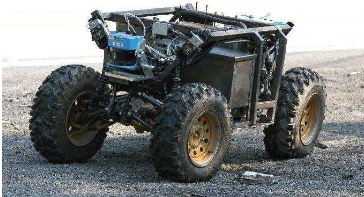
Figure 2-1: The Groundhog robot is a 1,500 pound custom-built vehicle equipped with onboard computing, laser range sensing, gas and sinkage sensors, and video recording equipment. [6]
