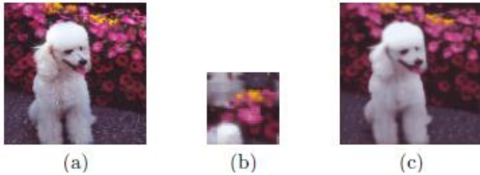
Figure 2-14: Appearance epitome: The input image (a), is epitomized in the texture (b), shown enlarged two times. The reconstructed image is shown in (c). [22]
