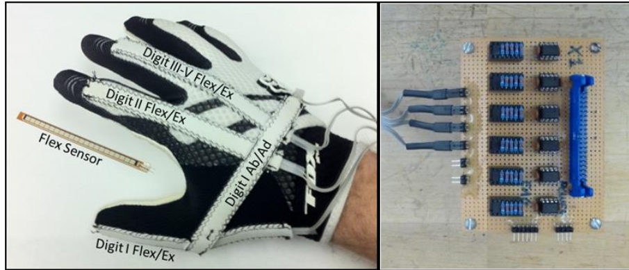
Figure 4.2 -The data glove used to capture motion of the native hand. Four sensors are used to capture flexion and extension of digits I-III, as well as abduction and adduction of the thumb. An individual flex sensor is also shown.
