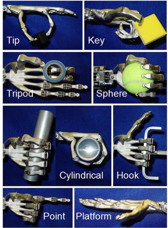
Figure 2.6 - Eight canonical hand postures, which constitute one of the primary design objectives of the hand prototype.
