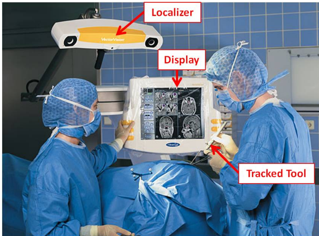
Figure II.7: Example of an image guided surgery setup showing an optical tracking system, tracked tools, and preoperative images displayed on a computer screen (image adapted from [12]).
