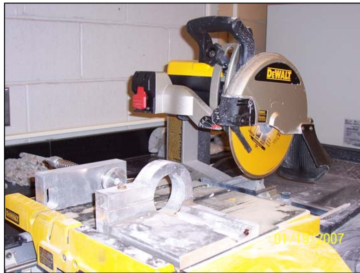
Figure 22. Tile Saw for Cutting Aggregate Plates
