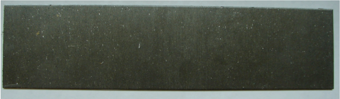
Figure 18 Sample of as-received Mg AZ31B. Sample is 3"x9"x0.09" The coating on the material prevents the Mg alloy from reacting with the environment.
