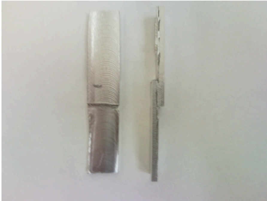
Figure 21: AZ31B machined to match the dimension of the tensile specimens for a baseline comparison.
