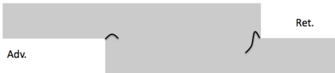
Appendix Figure 3. Drawing of the hooking defect observed in lap welds of Mg AZ31B. The black lines represent the hooking defect. This defect creates a stress concentration.
