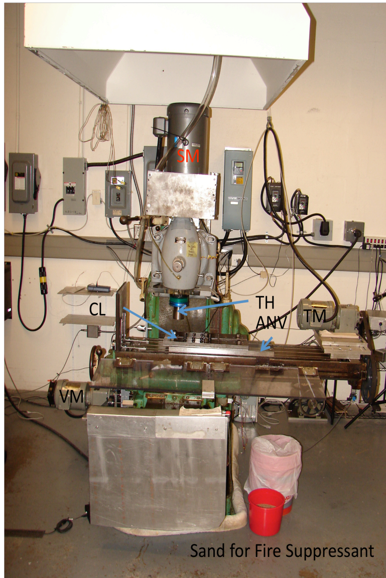
Figure 14 FSW Machine. CL: Clamps, TH: Tool Holder, ANV: Anvil, TM: Traverse Motor, VM: Vertical Motor, SM: Spindle Motor
