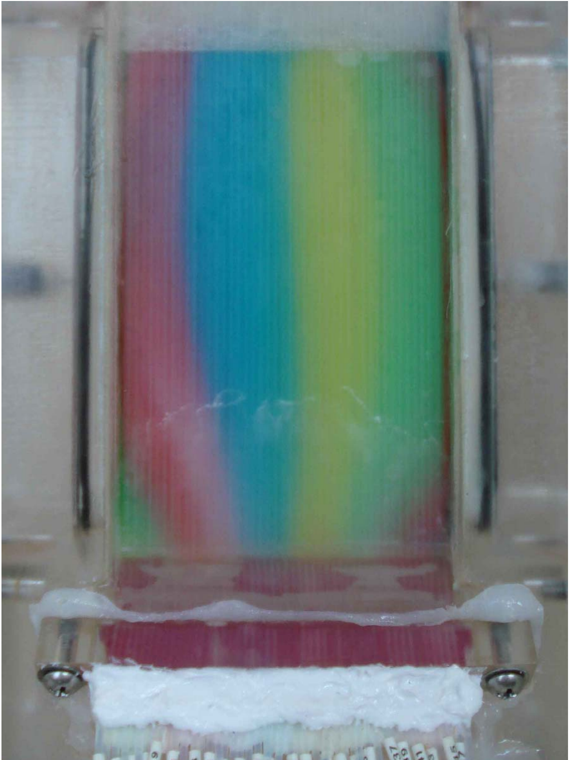
Figure A5. Picture of CFFE experiment checking the flow profile of solution inside the chamber. Here, flow of solution appears as uniform bands flowing straight down the chamber with no clear areas.
