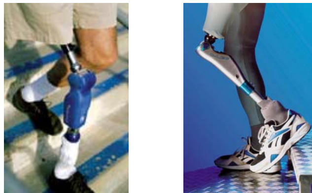
Figure 1-2. The Ossur Rheo knee (left) and the Otto Bock C-Leg (right) represent the cutting edge of microprocessor controlled damping prosthetic knees.
