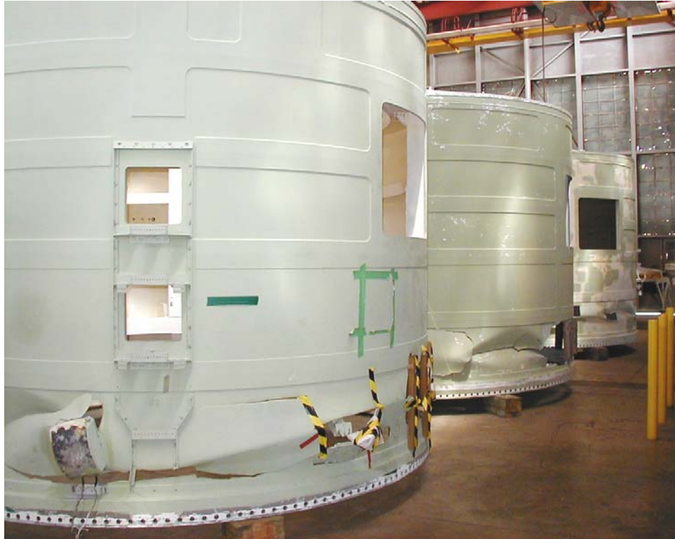
Fig. 5.9 – Three damaged SRB forward skirts
