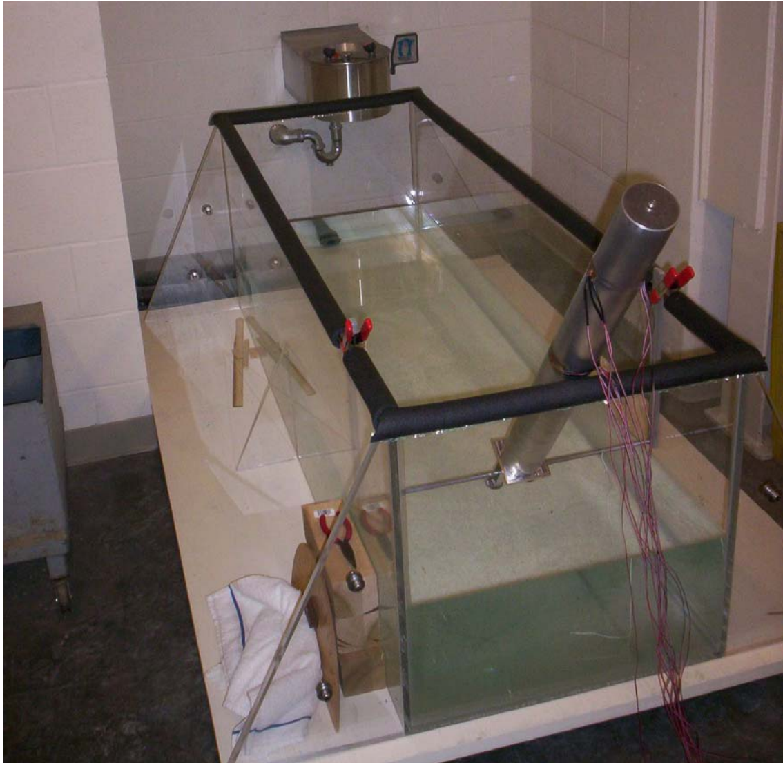
Fig. 4.2 – Experimental drop tank and hinged cylinder setup
