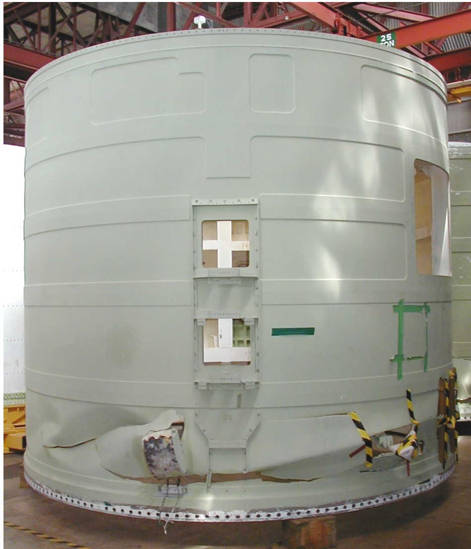
Fig. 5.1 – SRB forward skirt splashdown-induced damage
