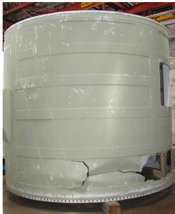
Fig. 1.2 – Damaged SRB forward skirt
