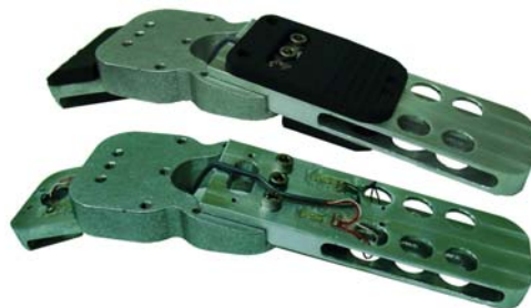
Figure 2-5. Sensorized prosthetic foot with and without strain gage covers.
