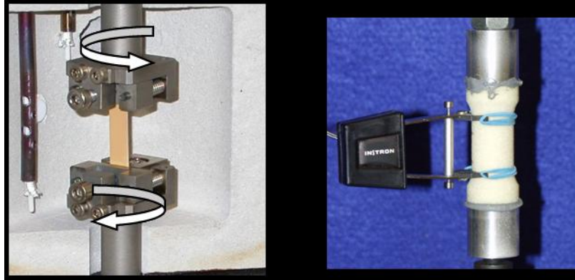
Figure 3.3. Torsional and tension experiments used for calibration
