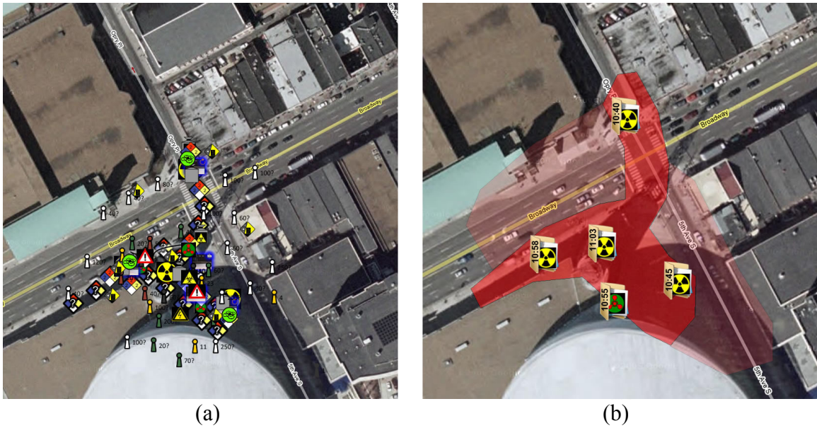
Figure 32: Two visualizations of information items: (a) the items are unorganized, and (b) the items are filtered and merged based on the CIFA results to support the hazard identification task.
