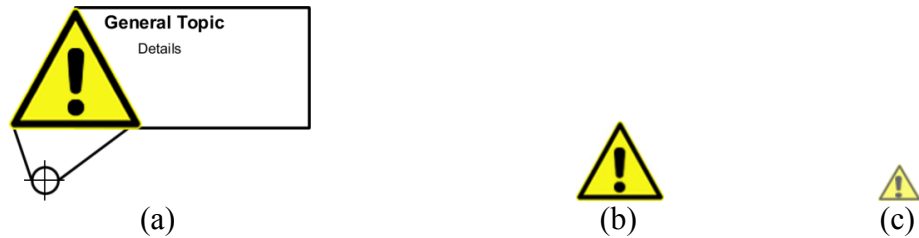
Figure 33: An example of the three visible information item visual states a) high detail, b) normal, and c) residue.
