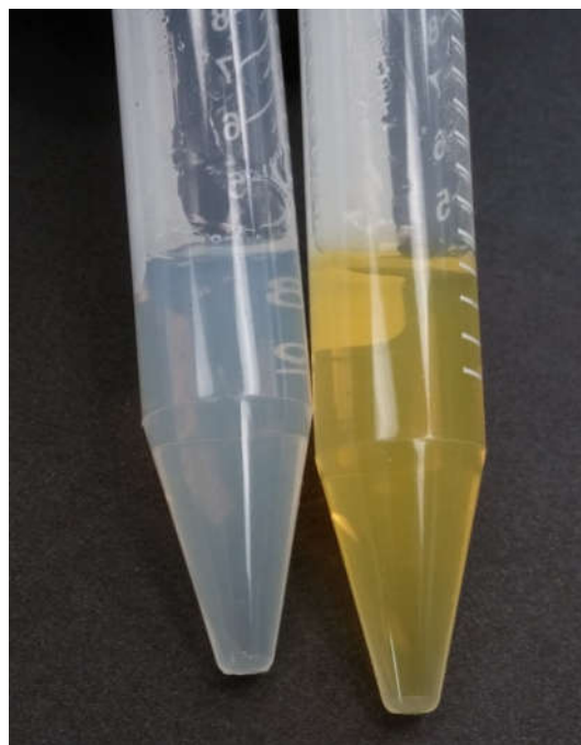
Figure 2: Comparison of a control hydrogel (left) with a hydrogel containing 0.001% ADA (right).
