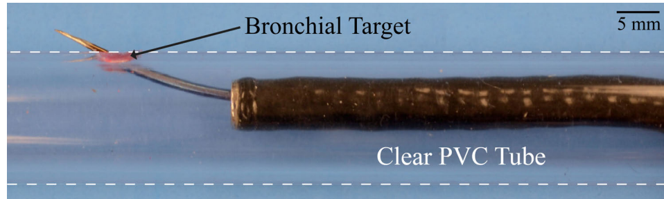
Figure 4.4: The concentric tube robot coupled with the tendon-actuated bronchoscope provide flexibility in selecting the position and orientation of the bronchial wall opening. This added dexterity also assists with orienting the initial pose of the steerable needle. Here, the bronchoscope and concentric tube robot are deployed in a clear PVC tube to a desired bronchial target on the wall of the tube.
