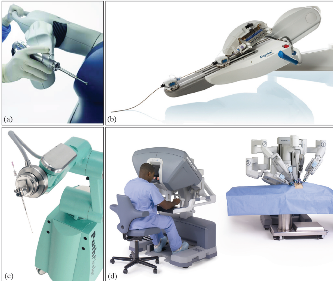
Figure 1.1: (a) The RIO orthopedic surgical robot. ©2015 Mako Surgical Corp. (b) The SENSEI robotic catheter system ©2015 Hansen Medical (c) The Pathfinder neurosurgical robot ©2012 ProSurgics, Inc. (d) The da Vinci laparoscopic surgical robot. ©2015 Intuitive Surgical, Inc.
