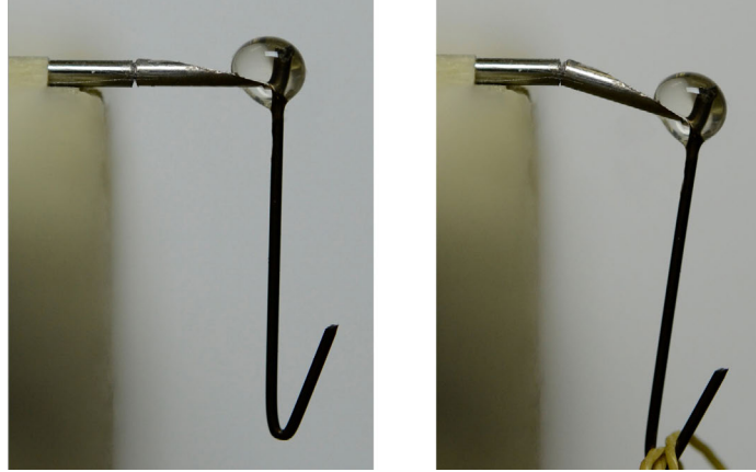
Figure 2.2: Experimental flexure stiffness test setup.
