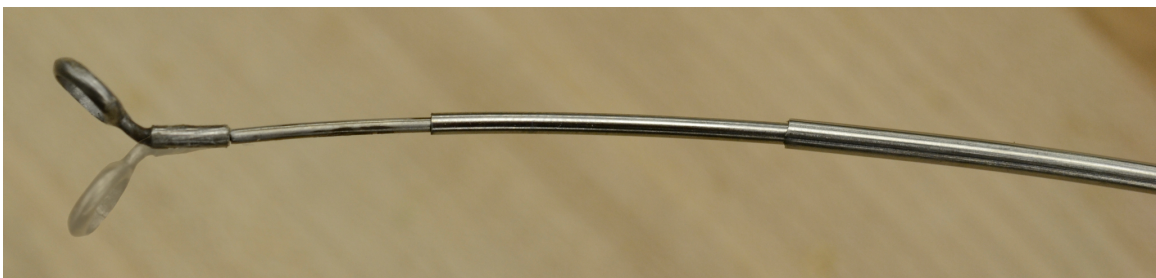
Figure 5.9: The ability to rotate the ring curette axially while the robot arm remains stationary is illustrated in this image via a semitransparent overlay of a second configuration of the curette.
