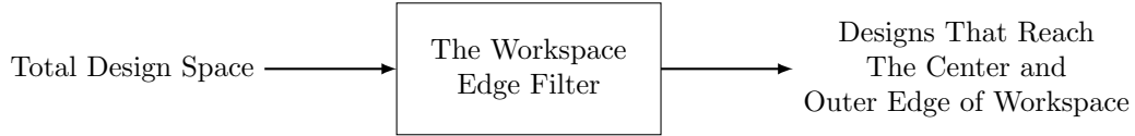
Figure 5.20: The basic input/output function of the workspace edge filter is shown. The input is a potential design space, and the output is a subset of designs that stably reach the center and outer edge of the workspace. This filter is numerically efficient because, since the structure is torsionless, the kinematics can be computed without the numerically expensive integration steps.
