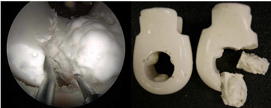
Figure 2.19: (Left) The left manipulator retracts the tissue, exposing the targets for the right manipulator to cut with the holmium laser. (Right) A photograph of what the prostate model looked like before and after the experiment.
