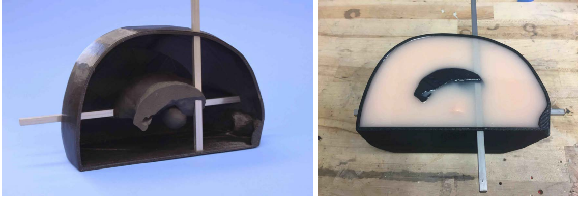
Figure 5.25: (Left) The assembled 3D printed skull and ventricle mold. (Right) The mold with the poured silicone while curing.
