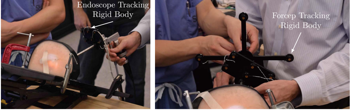
Figure 5.30: (Left) The endoscope/trocar inserted into the phantom. (Right) The endoscope/trocar inserted into the phantom with the forceps passing through the working channel. The forceps were under the control of the neurosurgical fellow and the endoscope was guided by the neurosurgeon.
