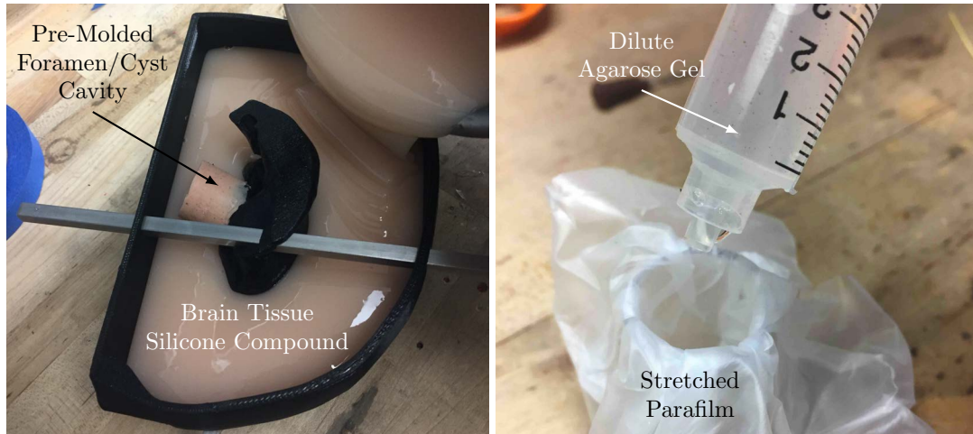
Figure 5.26: (Left) The brain tissue silicone is poured with the ventricles assembled using the square rods, and the foramen/cyst cavity already pre-cast out of stiffer silicone. (Right) Cyst preparation: the stretched parafilm is placed over a tube and a syringe is filled with a dilute agarose gel mixture. A string ties off the stretched parafilm to form the spherical cyst and act as the fibrous stalk attachment.
