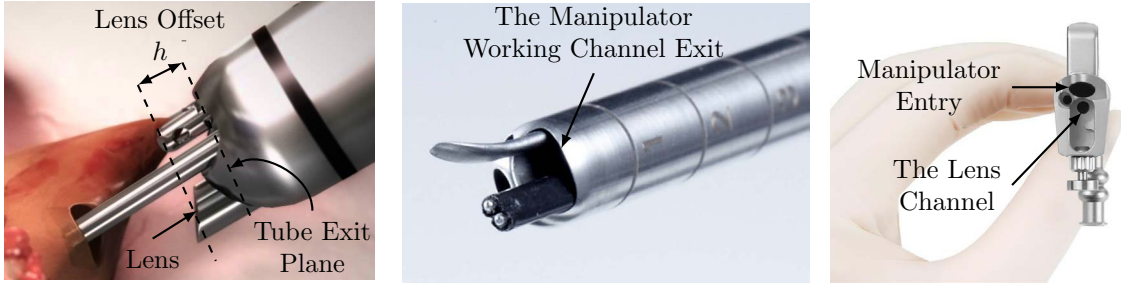
Figure 5.12: (Left) The lens offset is shown on the Aesculap Minop Invent. (Center) The distal tip of the endoscope’s working channel is shown. (Right) The proximal end of the Minop Invent is shown – the concentric tubes enter through the large elliptical working channel. [136].
