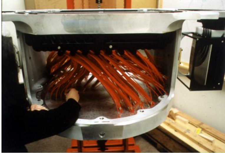
Figure 1.7 An image of a plug plate and cartridge used in SDSS. The optical fibers are plugged by hand into the plate (bottom) and lead to the spectrograph. The cartridge is slid behind the focal plane of the telescope to collect light from distant galaxies.
