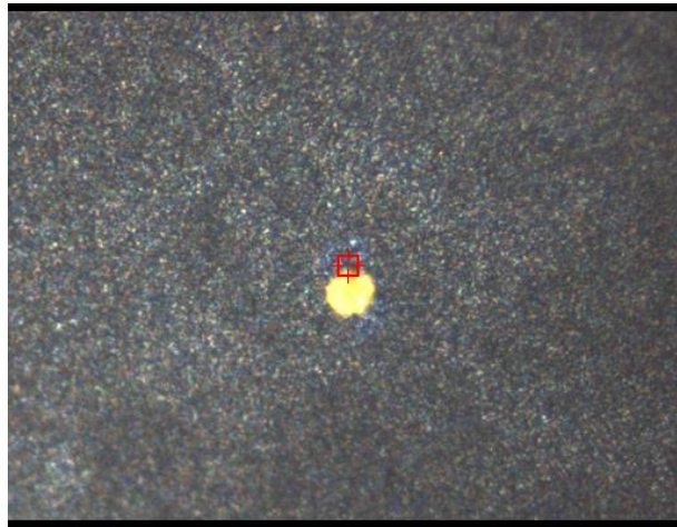
Figure 4.7 VO 2 particle film after laser irradiation, revealing oxidation of the sample area.
