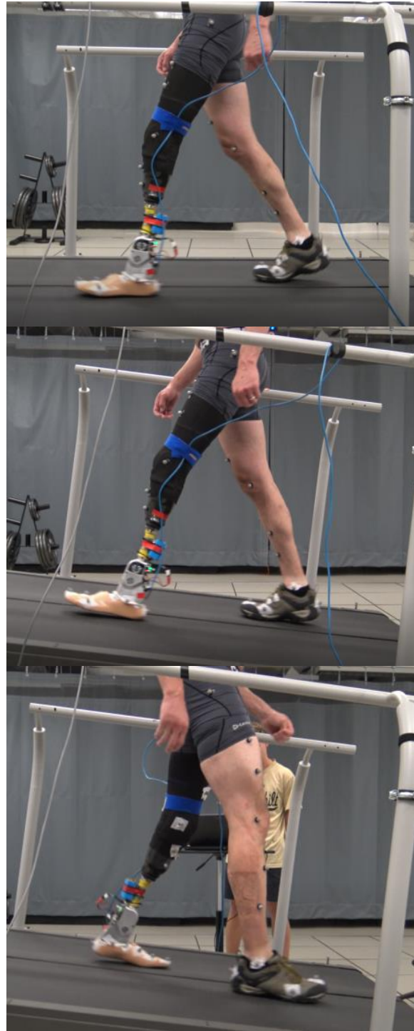
Figure 5. Participant walking with motion capture markers on instrumented treadmill at all three slopes
