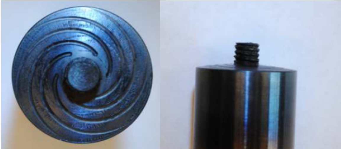
Figure 119 Spherical shoulder tool used for panel welds. Left image is a closeup of the spherical shoulder (with scrolls). Right image shows the tool in profile [127].
