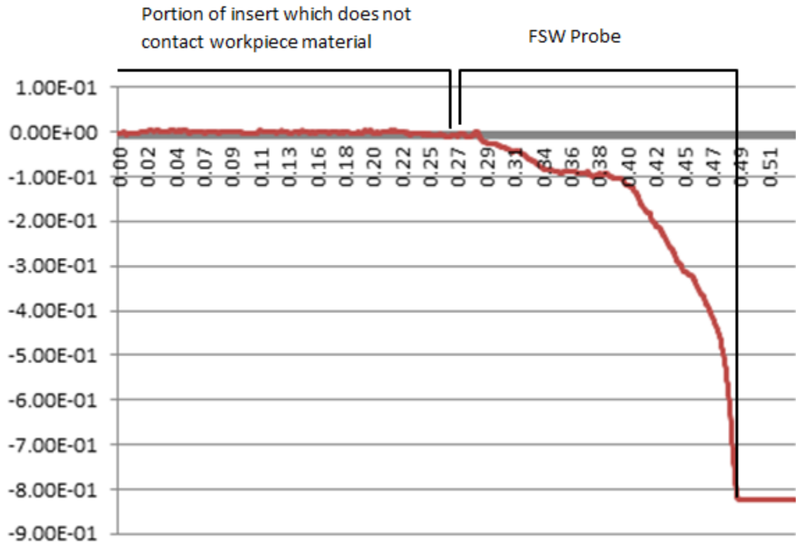
Figure 98 Plot of straight-line trace along the crest of a probe insert used to join Al 6061 containing F60 SiC at 1500 RPM and 5 IPM. The x axis represents the linear position
