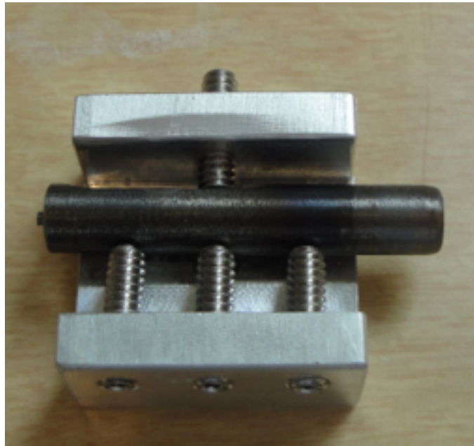
Figure 93 Probe insert mounted in specimen holder for imaging
