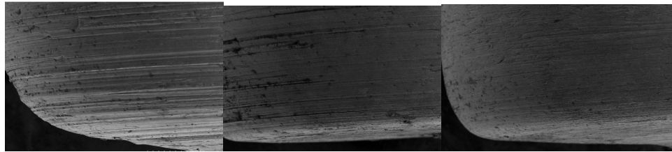
Figure 95 Post-weld images of probes used to join Aluminum containing (from left to right) F14, F60, and F150 SiC inclusions at 1500 RPM and 5 IPM.
