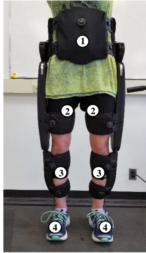
Figure 9. Photo of subject wearing the exoskeleton and IMUs. Numbers represent positions of Xsens IMUs at the pelvis (1); thighs (2), shanks (3), feet (4).
