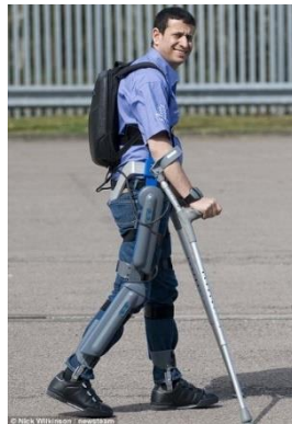
Figure 2. Photo of an individual using the a lower-limb exoskeleton that employs upper-limb user-balance-control.
