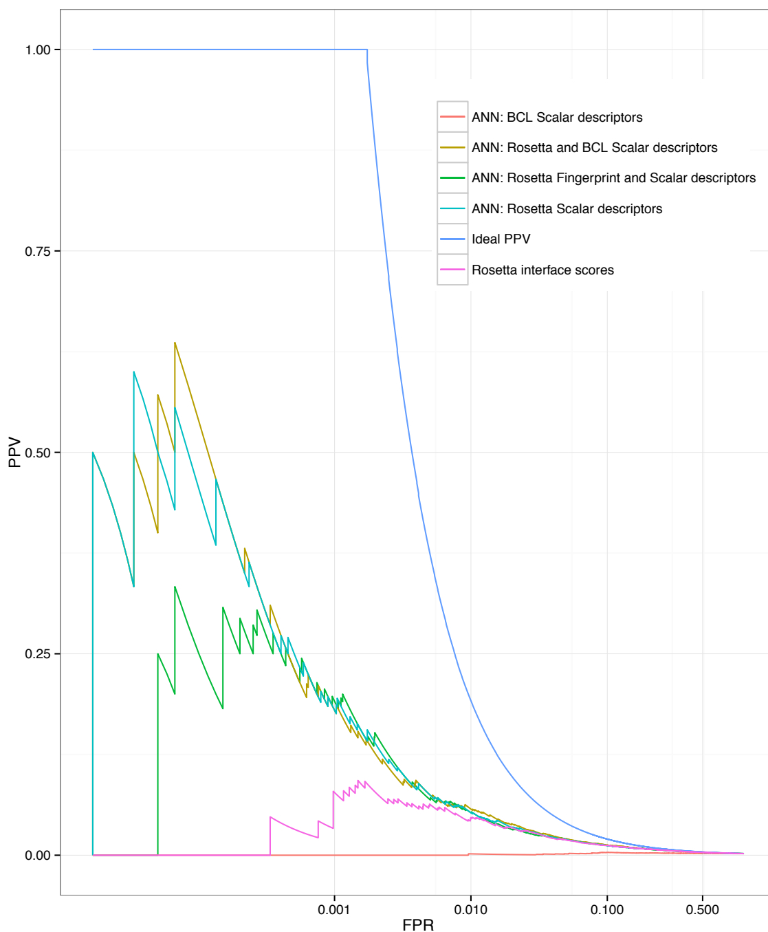
Figure IV.4: Plots showing the PPV as a function of FPR for the various networks trained using the 120 protein training set. Performance is plotted using the independent dataset from each of the 90 neural networks used. The PPV vs FPR curve of an ideal classifier is also plotted, for reference. To accentuate the differences in early classification, the X axis is plotted on a log scale.
