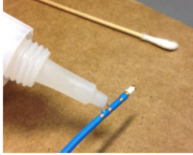
Fig. A.8 – Sealing ring electrodes near tip with cyanoacrylate adhesive to prevent nitrous oxide gas leakage.
