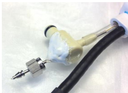
Fig. A.5 – New cryo delivery tube and vacuum connector completed with compression fitting components.
