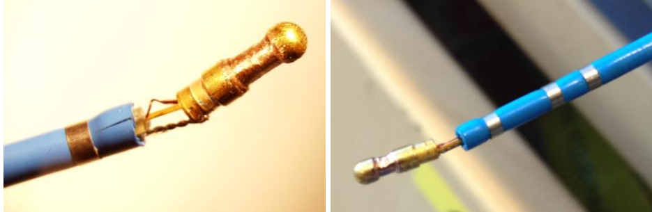
Fig. A.6 – Catheter tip prior to being glued to the distal catheter body.
