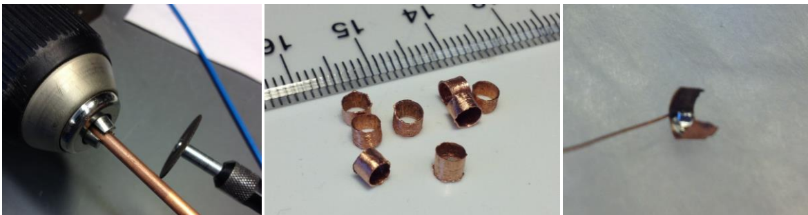
Fig. A.9 – Left: Drill-Dremel lathe setup for reducing the OD of 4mm diameter hollow copper rod. Center: Completed RF electrodes. Right: RF electrode cut lengthwise with RF wire soldered.
