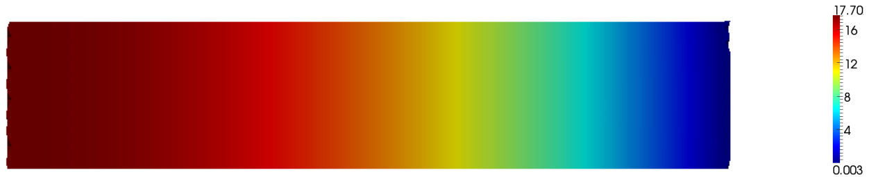
Figure VII. 8: These are the pressure and displacement solutions when 100 Pa was applied to the left hand side of the column, and it was specified that the pressure and displacement on the right hand side of the column is 0. This rectangular mesh was unsplit. Warm colors represent higher pressure and displacement values, while cooler colors represent lower pressure and displacement values.
