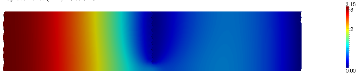
Figure VII. 10: These are the pressure and displacement solutions when 100 Pa is applied to the left hand side of the column, and it was specified that the pressure and displacement on the right hand side of the column is 0. This rectangular mesh was split, and the split is fixed in displacement. Warm colors represent higher pressure and displacement values, while cooler colors represent lower pressure and displacement values.
