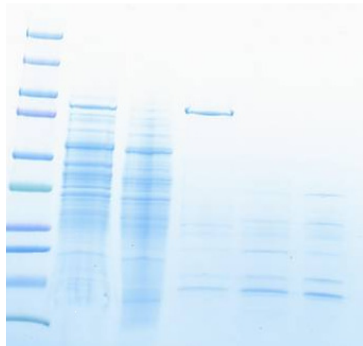
Figure 4-15. SDS-PAGE analysis of NAT purification. (lane1: marker, lane2: streptomycin sulfate supernatant, lane3: 75%AS pellet resuspended and dialysed, lane4: Q-sepharose active fractions, lane5: DEAE-sepharose active fractions, lane6: monoQ active fraction)
