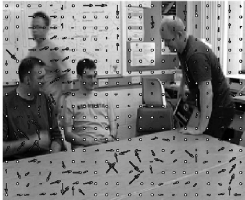
Figure 2:25: 16x16 motion vectors (superimposed on frame).
