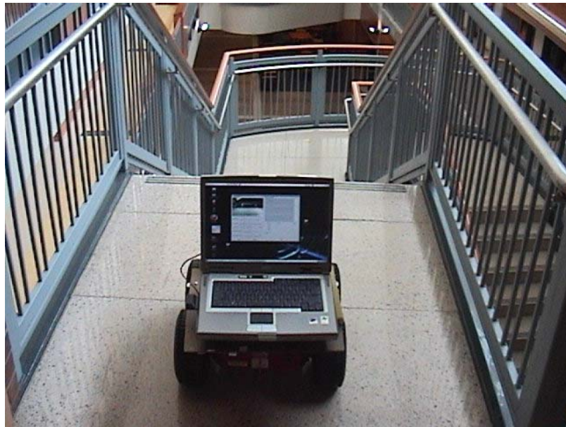
Figure 7.18: Mobile robot detecting real precipice.
