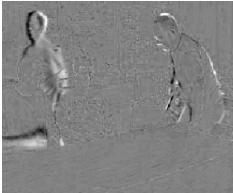
Figure 2.24: Residual F_n - F'_{n-1} (no motion compensation).
