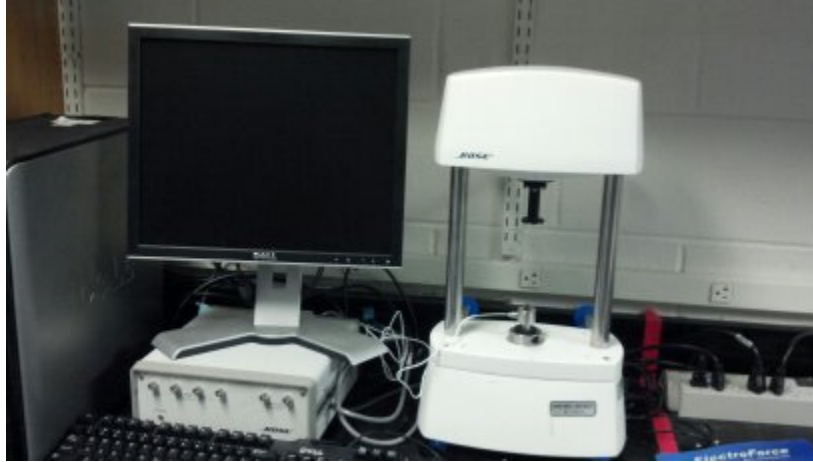
Figure 15. Mechanical tester (right) and workstation (left) which are used to obtain material properties of phantom samples to validate strain imaging.
