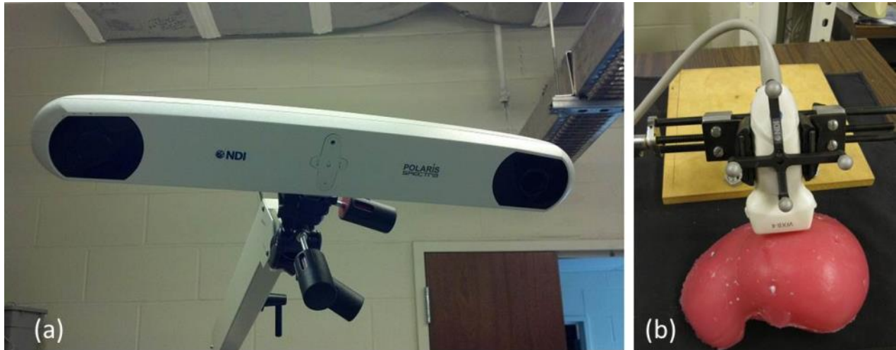
Figure 37. The tracked ultrasound system consisted of a Polaris optical tracking system (a) and a passive target attached to the ultrasound probe (b).
