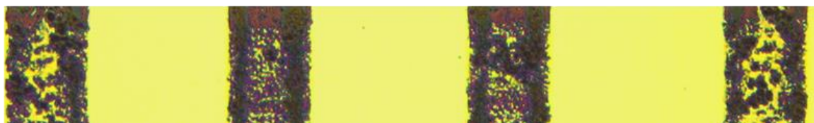
Figure 4.5. Optical images of 100 \mu\text{m} -wide crystal violet lines after MALDI imaging. (a) Effect of operating in an overlapping mode where a moderate laser power was used. (b) Effect of operating in an oversampling mode where a high laser power was used.
