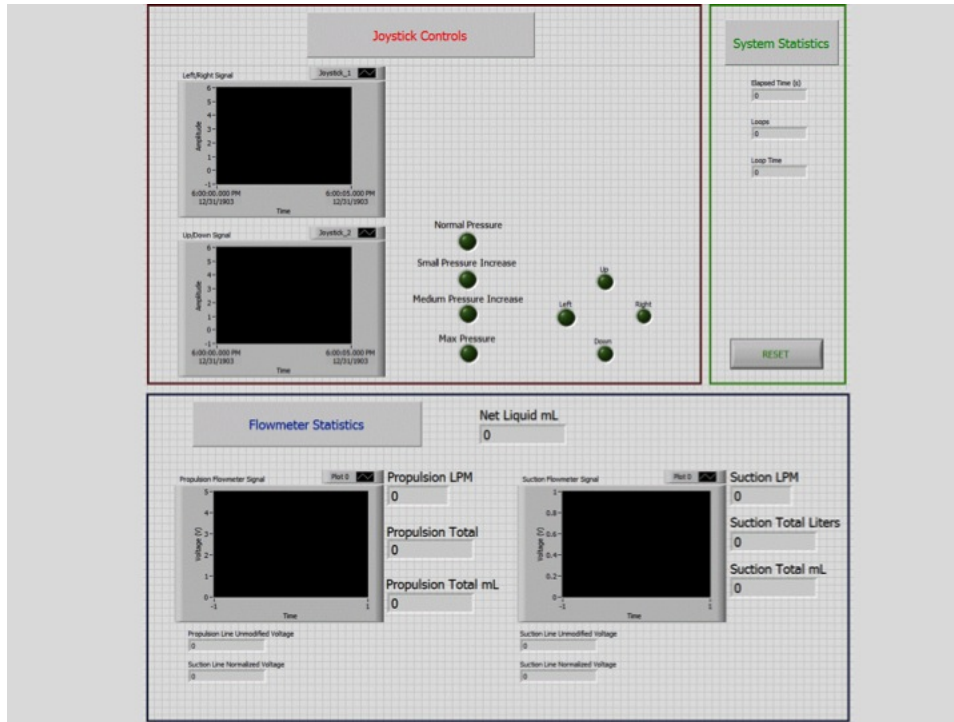
Figure 3.3: Image of the LabView Based Graphical User Interface for the Hydrojet System
