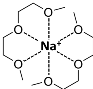
Figure 6: Illustration of a Na ion coordinated to two diglyme molecules.
