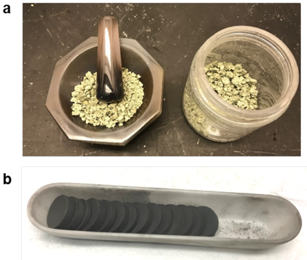
Figure 44: (a) Dried precursor after ball milling. (b) Sintered \text{Na}_3\text{V}_2(\text{PO}_4)_3 discs in ceramic boat.
