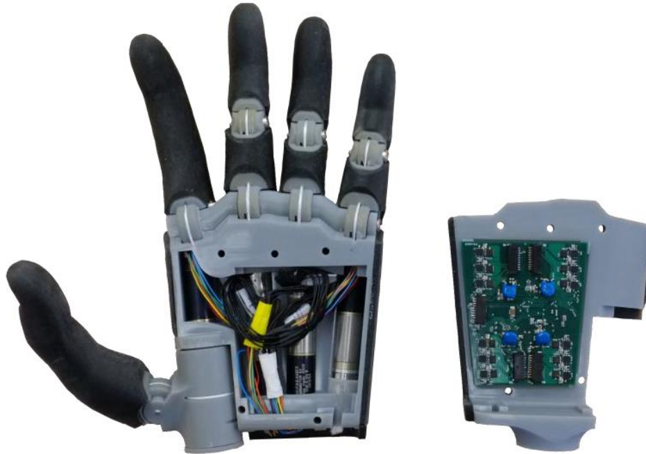
Fig. 2 VMG with the embedded control system
