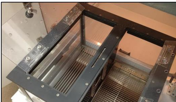
Figure 9. Apparatus used for GluN1 -/- conditioned place preference experiments. To minimize variability, cocaine was always paired with the side with bar floors (left) while saline was paired with the side with grid floors (right).
